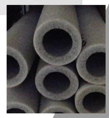
Low density polyethylene closed cell foam 40-50kg/m3 nominal
