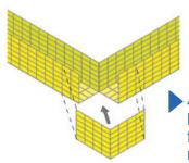
4. Suitable for High Speed Formwork - Pecafil is designed for fast assembly. No hammer, nails or saws, just tie wire.
